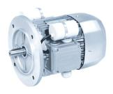
Single-phase motors of the BS series are manufactured to the applicable IEC standards and are of the enclosed type, externally ventilated and with run capacitor permanently connected. Motors are available in the B5 and B14 flange mountings, in the 4-pole execution. For applications requiring high starting torque the version with both the run and the starting capacitor can be specified.
