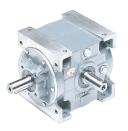
The units of the RAN series are designed to fit the purpose of transmission laid out in right angle setting. Easy to fit and almost maintenance-free, RAN units offer multiple shaft arrangements and a choice of several exact gear ratios, beside the 1:1, that come handy when designing synchronized drive system. Also available in the version for screw jack duty.
